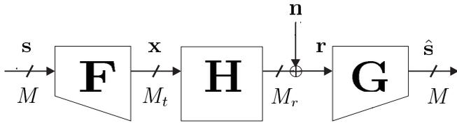
**Fig. 1.** A MIMO system with  $M_t$  transmit antennas and  $M_r$  receive antennas.
