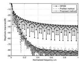
Figure 3: Magnitude response of the transmit prototype filters.
