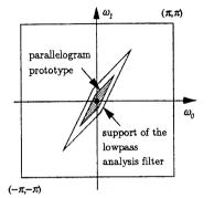
Fig. 7. Simplistic four parallelogram filter bank. The parallelogram prototype  $SPD(\pi N^{-T})$  and the support of the lowpass analysis filter  $SPD(\pi M^{-T})$ .
