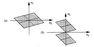
Fig. 6. Two of the possible supports for the 0th analysis filter.
