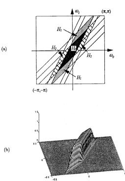
Fig. 10. Example 4.1. Simplistic four-parallelogram filter bank (a) Spectral support of the analysis filters and (b) the magnitude response of the lowpass analysis filter with frequency normalized by  $2\pi$ .
