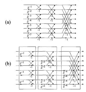
Figure 2: (a) An implementation of  $H\Lambda(z)$ . (b) An equivalent system.
