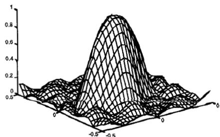
Fig. 6. Example 4.1. Two-dimensional linear phase cosine modulated filter bank. The magnitude response of the prototype with frequency normalized by  $2\pi$ .
