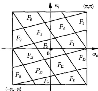
Fig. 4. Example of a 2D DFT filter bank.
