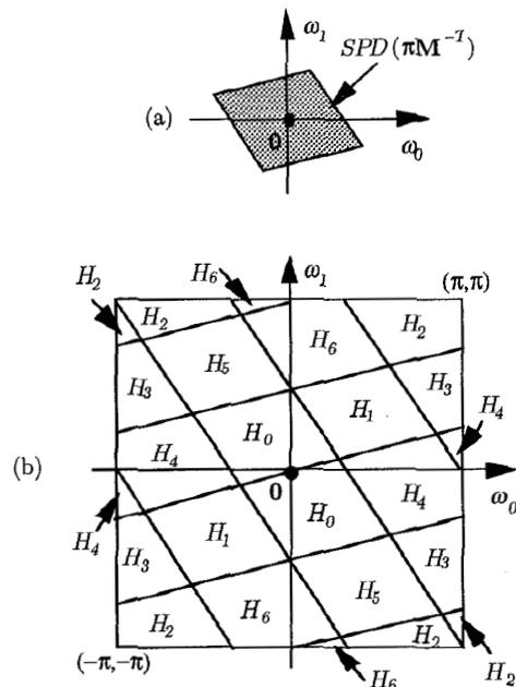
Fig. 2. A typical two-dimensional cosine modulated filter bank, (a) spectral support of the prototype, (b) support configuration of the filter bank.
