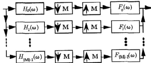
Fig. 1.  $|M|$ -channel maximally decimated filter bank, where  $|M| = |\det M|$ .
