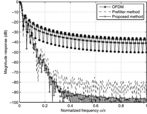
Figure 4: Magnitude response of the receive prototype filters.
