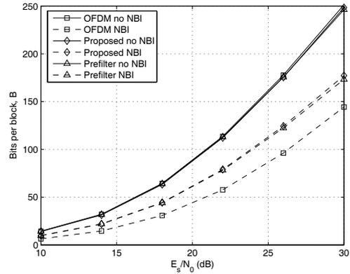
Figure 5: Comparison of bit rate.
