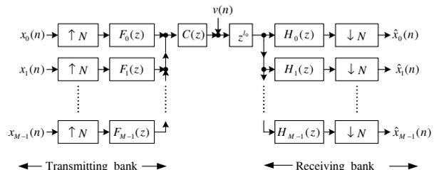
Figure 1: A filter bank transceiver.
