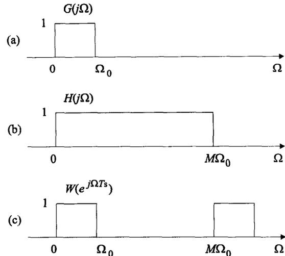
Figure 4: Example 2. Illustration of  $G(j\Omega)$ ,  $H(j\Omega)$  and  $W(e^{j\Omega T_s})$ .
