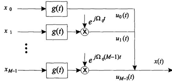
Figure 1: The baseband analog representation of the OFDM transmitter with  $M$  subcarriers and pulse shaping filter  $g(t)$ .
