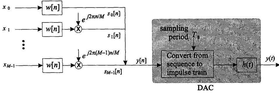
Figure 2: Commonly used digital implementation of the OFDM transmitter.
