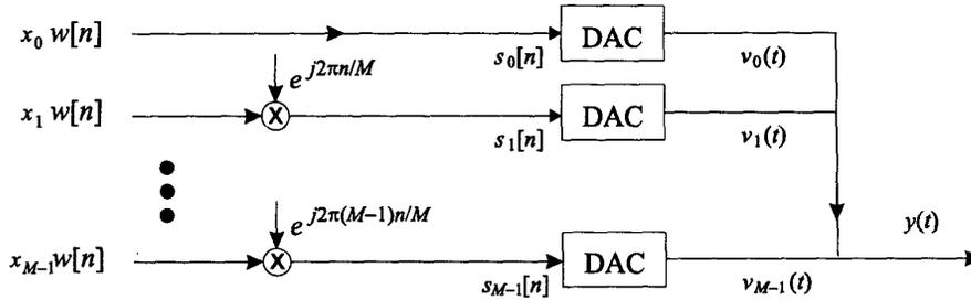
Figure 3: Equivalent block diagram of system in Fig. 2.
