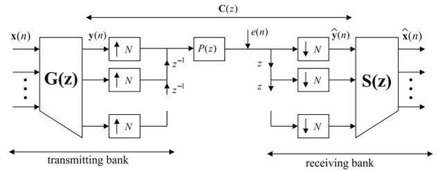
Figure 2: The polyphase representation of the transmitter and receiver in a filterbank transceiver.
