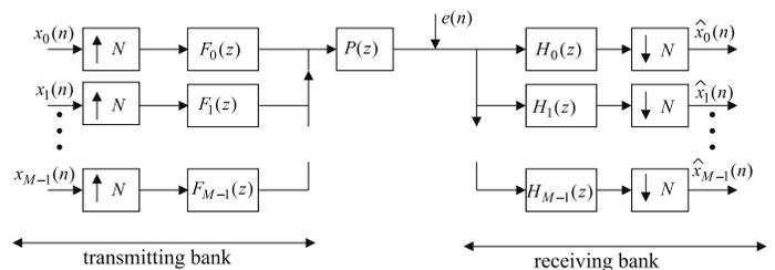
Figure 1: An  $M$ -subband filterbank transceiver over a non ideal channel  $P(z)$ .
